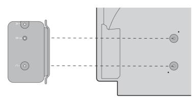
The screw holes and guide pins shown on the back of LCD Projection TV with the bracket (holes B and C) for left side attachment.
